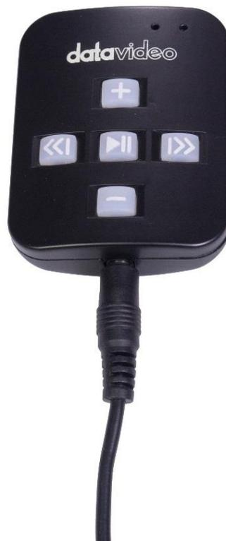
**NOTE:** When using this remote in wired mode the **DV Prompter app** should also be set to **Wired – WR-500** in the **Remote menu option**.
